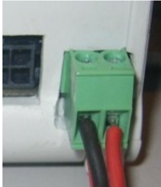
Picture 5 – Power supply terminal block
