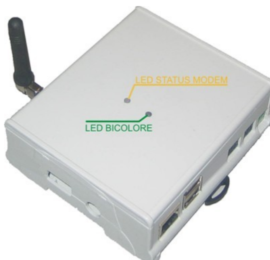
Picture 10 – Signalling LEDs
